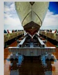
A ship lift is a controlled platform that lifts and launches a ship and transfers it onto land. The platform can be controlled from a control desk in a tower to provide the operator with a thorough view of the entire operation.
